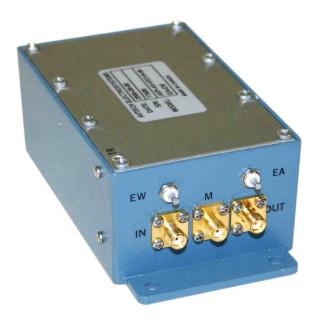
AVP-AV-HV3 units also have a "TR" trimpot accessible from the top cover, The "TR" control is a ten-turn trimpot which varies the output rise time and pulse top flatness. For PRF below 200 kHz (approximately), this control is normally set fully counter-clockwise. For higher PRF the control may need to be set fully clockwise for best performance. The AVP-AV-HV3 is shipped with this control the fully counter-clockwise position.
